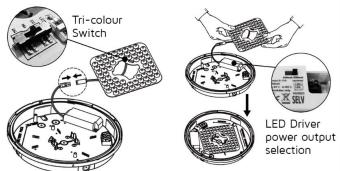
Step 7: Attach the Diffuser to the Housing Base, then rotate Then attach the LED Gear Tray Bulkhead Base. Select the required clockwise to lock in position and align fixing holes for anti-tamper screws. Install the 2x diffuser anti-tamper screws provided.
