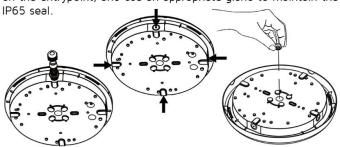
Step 4: Install the Bulkhead Base using the included fixing screws. Step 5: Wire the Gear Tray as per the diagram below.
