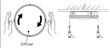
Step 8: Attach the Outer Ring to complete the installation.
