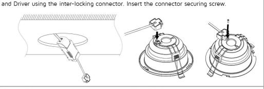
Step 2: Wire the LED driver to the mains supply junction box. Connect the Downlight
